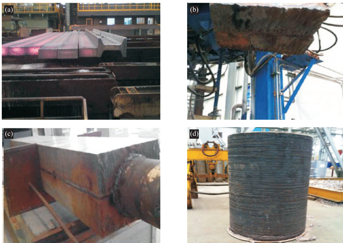
Fig.1. The production of H13 ESR_CC tool steels: (a) CC bloom (200×480mm), (b)Auto slag feeding, (c)Electrode assembling and (d)3t ingot.
