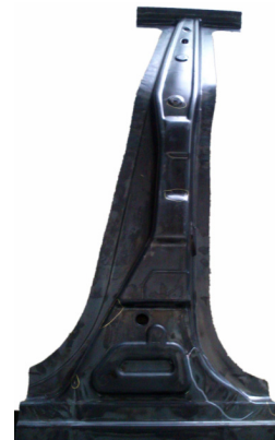
Fig.7. The photo of hot stamped B pillar with patchwork blank design.
